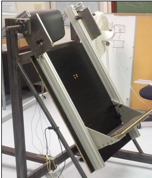
Figure 2.10: The foot rest can quickly be adjusted along the leg platform to accommodate a wide range of participant heights.
